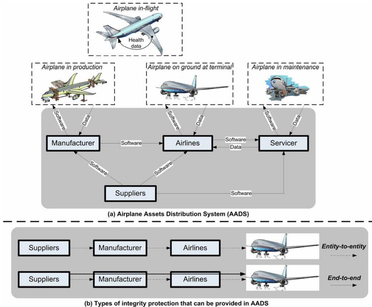
**Fig. 1.** (a) Distribution of signed assets during lifecycle of the airplane in the Airplane Assets Distribution System (AADS). (b) Illustration of entity-to-entity and end-to-end integrity protection in AADS.
